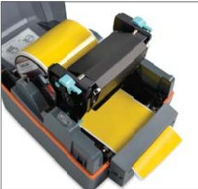
Feed the supply under the print carriage, threading it beneath the green adjustable label guides, and over the top of the rubber roller near the cutter module
