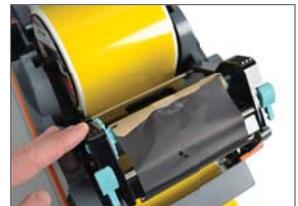
Loose end of the ribbon pulled up and around the print head carriage and secured to the empty rewind core.
