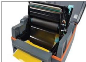
Ribbon core fitted in the holder on the underside of the print head carriage.
